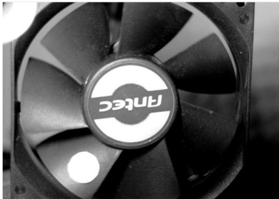
Picture 6 – Fan. Rotation speed 40 rps. Camera shutter 83  $\mu$ s. Diaphragm is fully opened. Zero gain. Strobe light impulse 90  $\mu$ s. EZSyncLed light.
