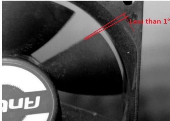
Picture 2 – Fan blade. Rotation speed 40 rps. Camera shutter 130  $\mu$ s. Diaphragm is fully opened. Zero gain. EZSyncLed light.
