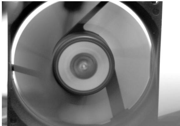
Picture 1 – Fan. Rotation speed 40 rps. Camera shutter 12ms. Diaphragm is fully opened. Zero gain. Regular fluorescent light.
